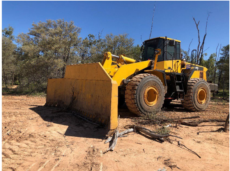
Above left. Geoff Urquhart describing the design of stick contours that have been effective in slowing water velocity and erosion. Above right. Machine used for stick raking.
